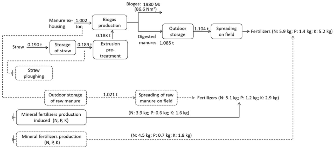
Figure G-2: System boundary considered for the inventory data of mono-digestion of fattening pig slurry. Dotted lines indicate an avoided process while full lines indicate an induced process.
