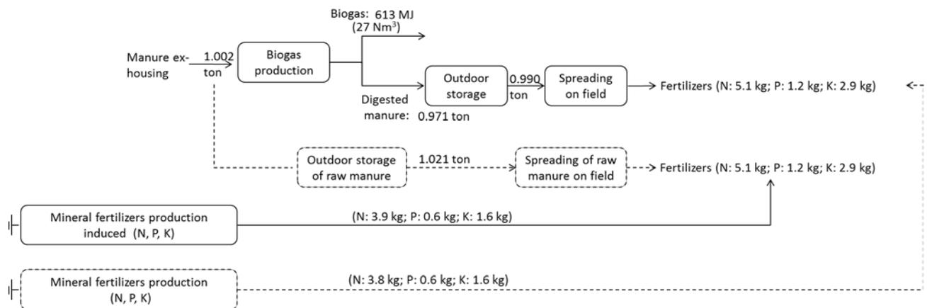
Figure G-1: System boundary considered for the inventory data of mono-digestion of fattening pig slurry. Dotted lines indicate an avoided process while full lines indicate an induced process.
