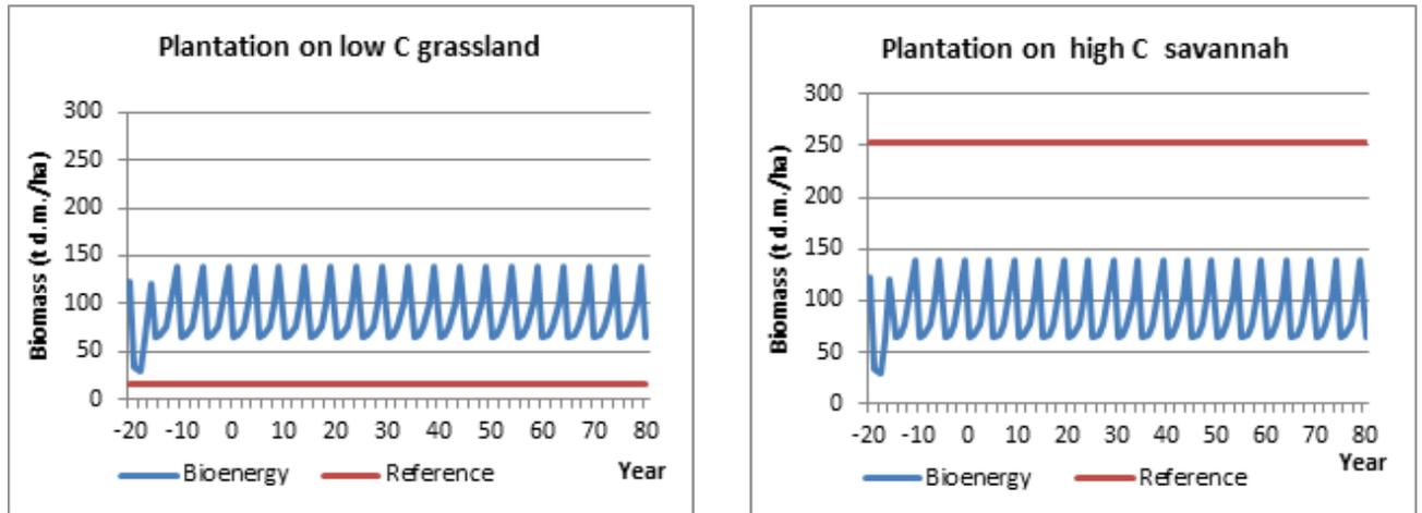
Figure 5 Changes in C-stock (biomass in ton dry matter (d.m.)/hectare) when establishing a plantation on low carbon stock grassland in the tropics versus on a high C woody savannah. Data, models and assumptions are presented in Appendices A to E
