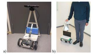
Fig. 1. a) The Intelligent Carrying Assistant Robot (iCAR) b) Humanfriendly walking assisting robot vehicle (hWALK).
