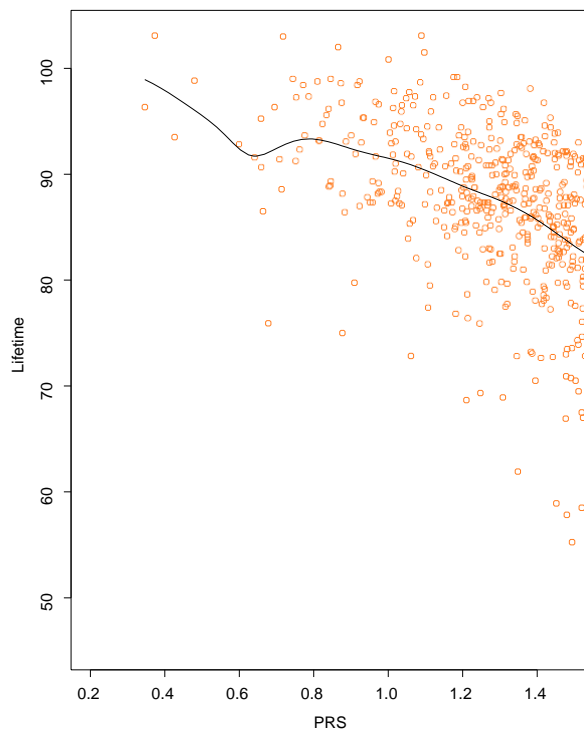
Figure 2: Plot of realized lifetime versus PRS by using only the uncensored observations from the whole dataset. The solid line represents estimated lifetime expectancy; it is obtained by local linear regression, where the Gaussian kernel is employed. The bandwidth is chosen according to the Silverman Rule-of-Thumb.
