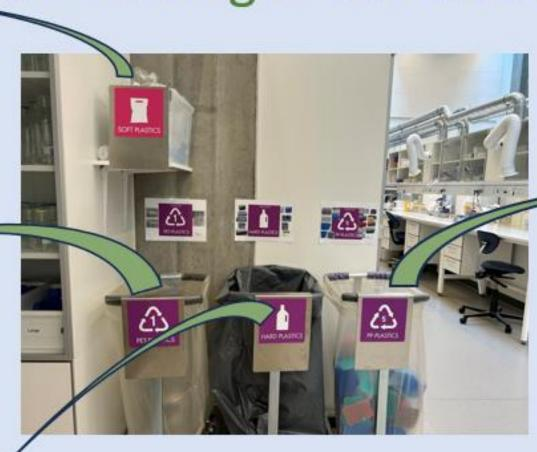
PP5 fraction is collected in the lab and technical service granulate it, before AVL picks it up and reuse PP5 for new products
