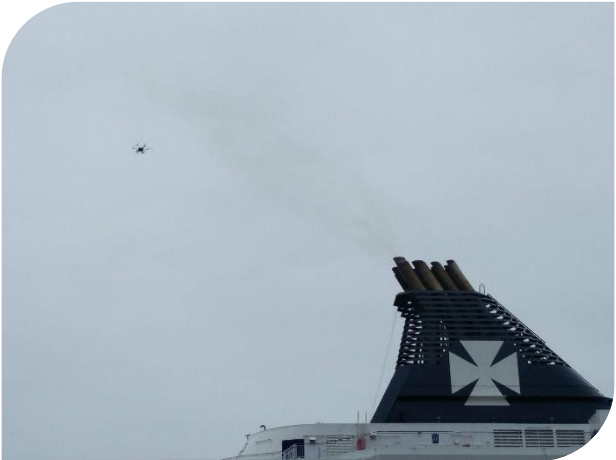
A drone positioned behind a ship's exhaust plume.
