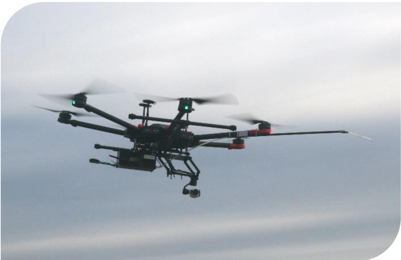
Explicit's mini sniffer system mounted on a drone.
