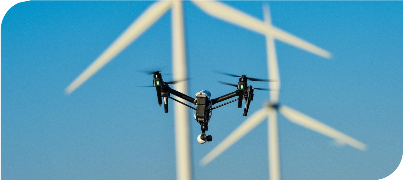
A drone on a wind turbine blade inspection mission.
