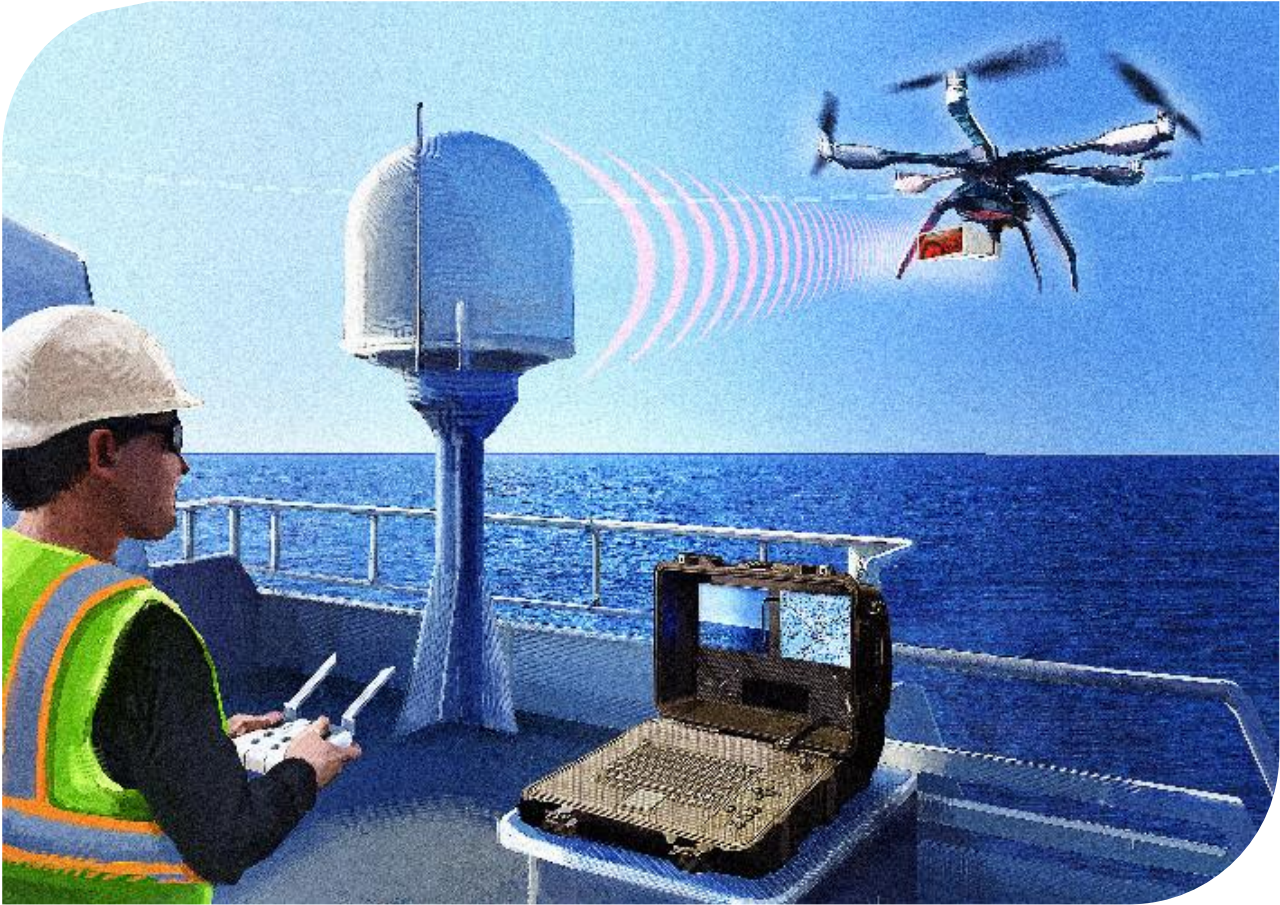
Illustration of QuadSAT's drone solution for testing ships' satellite communication systems.
