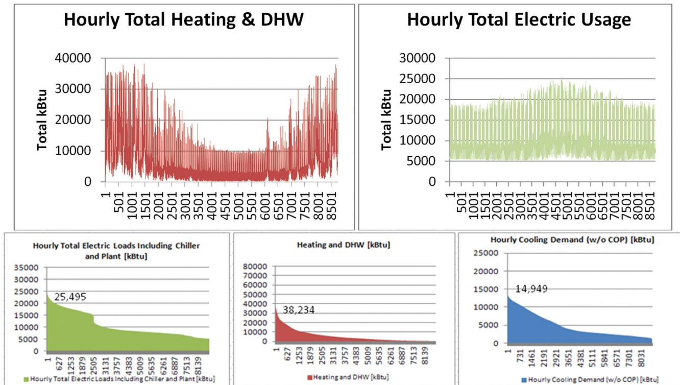
**Figure 6** Load profiles—new buildings built to EISA-ready specifications; all other buildings to Epact specifications.
