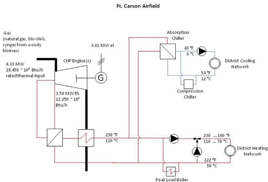
**Figure 8** Schematic alternative no. 2—CHP engines.
