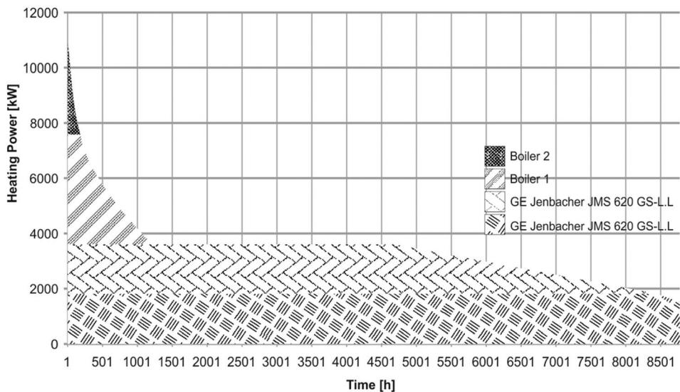
**Figure 9** Distribution of heating generation for alternative no. 2.
