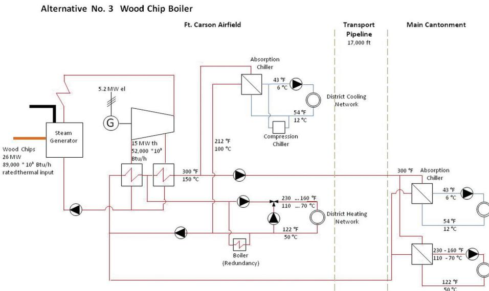
**Figure 10** Schematic alternative no. 3—wood chip boiler.
