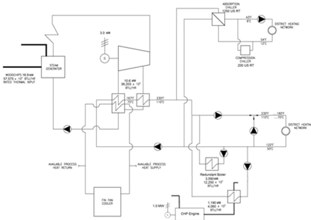
**Figure 11** Schematic alternative no. 4—wood chip boiler.
