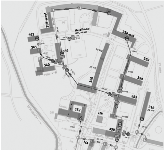
Figure 12 Measuring points in the heating grid of the NZE northern grid (image used courtesy of RK-Stuttgart Architecture and Energy Design).
