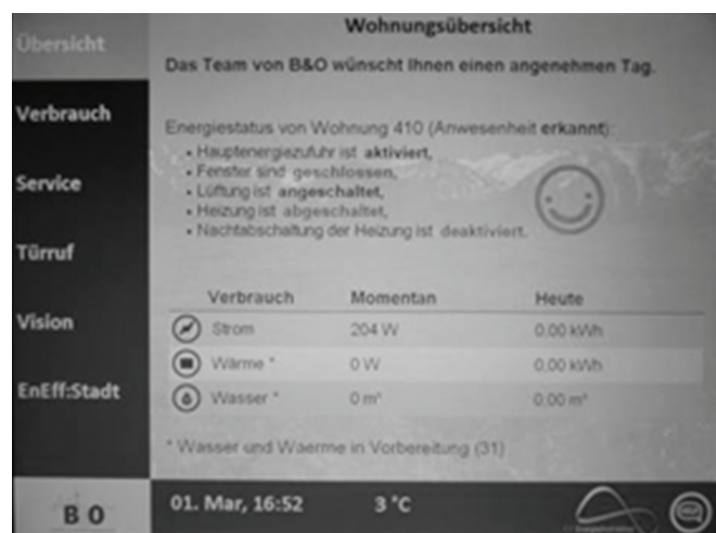
Figure 11 Smart metering displays help the tenants to get an overview of their energy and water consumption and the resulting costs (image used courtesy of RK-Stuttgart Architecture and Energy Design).
