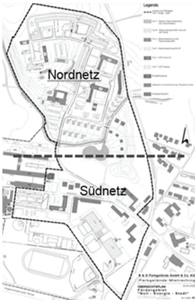
Figure 5 Separation of the district heating grid into a northern and a southern grid with different temperature profiles according to demand (image used courtesy of Schankula Architects).
