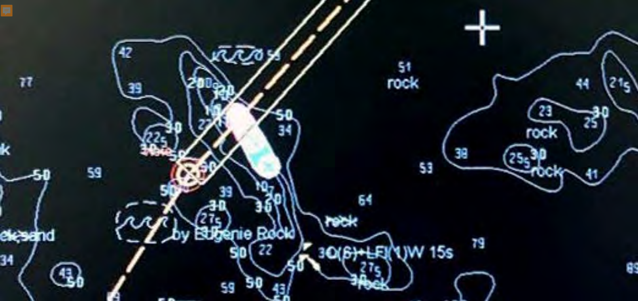
Kaami's route passing over shoal waters after WP 19. Photo from the ship's ECDIS. Courtesy MAIB.
