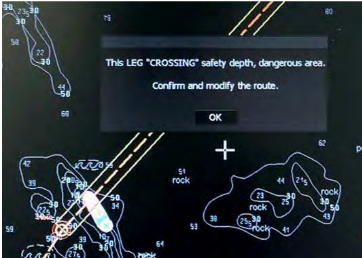
Figure 8: Voyage planning screen showing XTD and safety check. Voyage planning display screen with cross track limit and automatic safety check data highlighted. Courtesy of MAIB
