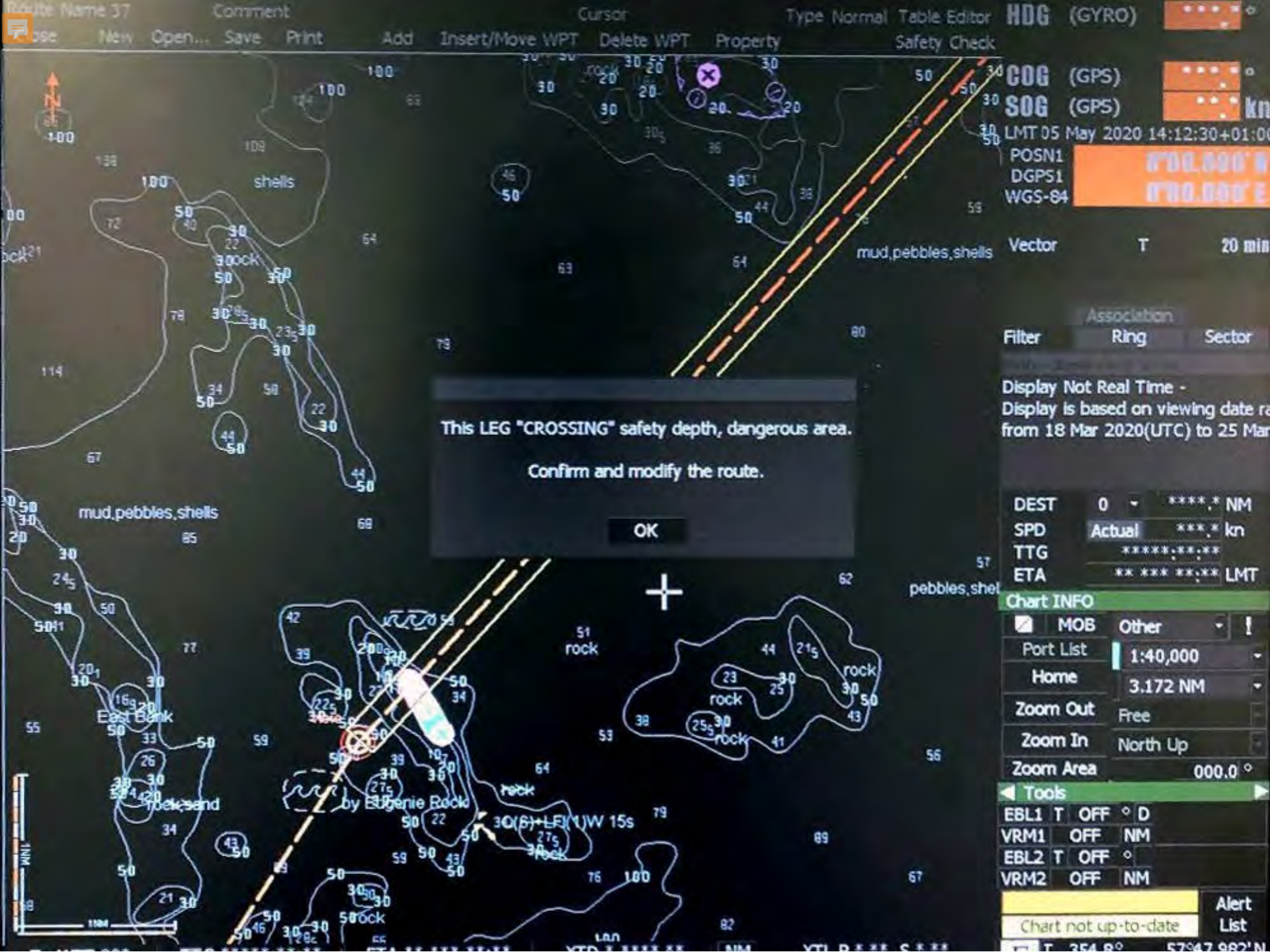
Figure 14: Automatically generated alarm for crossing a safety contour. Courtesy of MAIB
