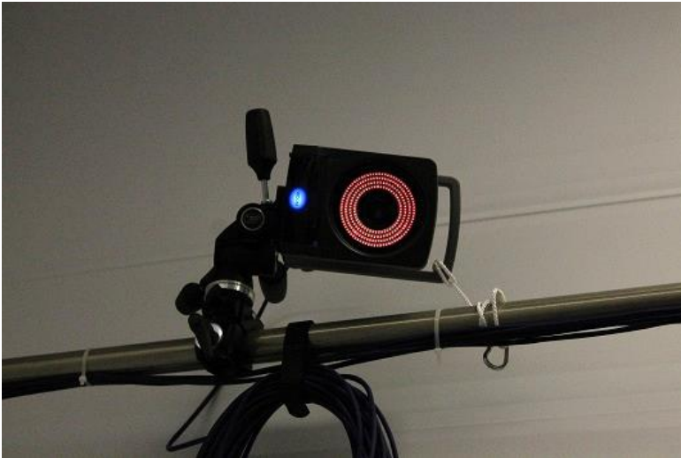
Figure 3: VICON camera (MX-T40s)
