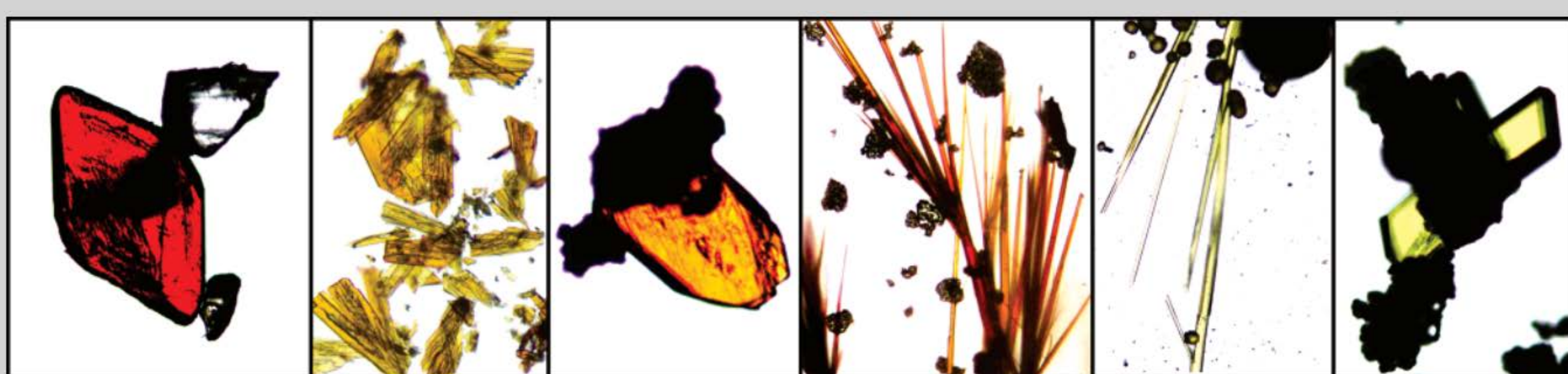
Figure 4. Photomicrographs of ROY polymorphs produced in the presence of polymers. From left to right: red prism (hydrolyzed poly(vinyl alcohol)), orange-red plates (acetoxystyrene/hydroxyethyl methacrylate/divinylbenzene terpolymer, not shown), orange plate (vinyl chloride/vinyl acetate/hydroxypropyl acrylate terpolymer), orange needles (ethylene/propylene copolymer), yellow needles (styrene/butyl methacrylate copolymer), and yellow prism (vinyl chloride/vinyl acetate copolymer).
