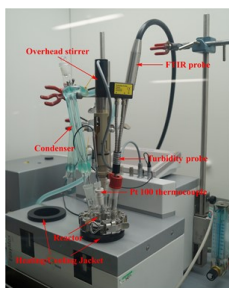
Figure 1: Experimental set-up for crystallization in lab-scale [5].
