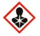
Health hazard/ Carcinogen/ Mutagen/ Reproductive toxicity/ Specific target organ toxicity/ Aspiration hazard/ Respiratory sensitiser
