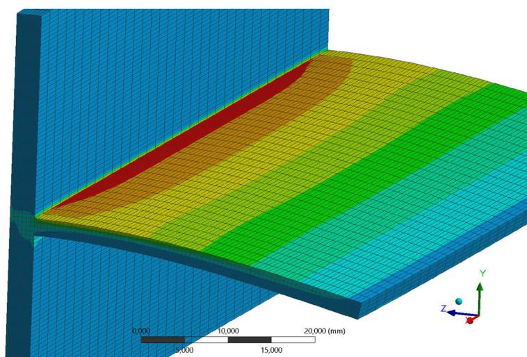
Figure 1: Distribution of maximum principle stresses in a specimen
