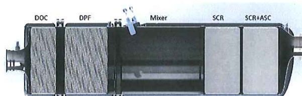
Figure 3. An inline EU-VI ATS with an open void where the Low Thermal Mass Compact Mixer is to be placed [7]
