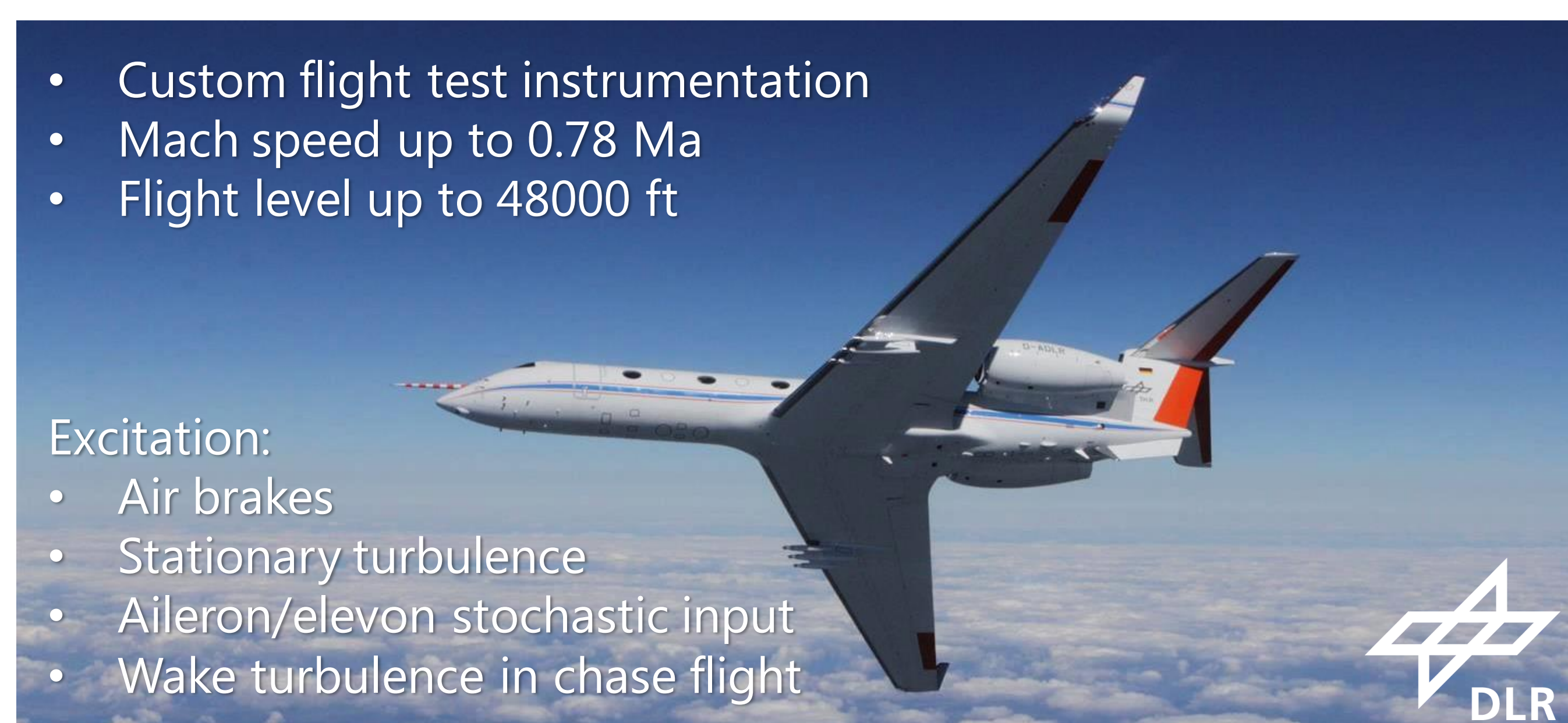
Figure 1: The DLR Gulfstream G550 HALO research aircraft and some features of the test campaign
