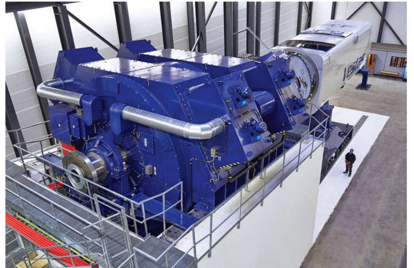
Figure 2: Function Test Bench installation at LORC, a Vestas turbine can be seen installed on the test bench.
