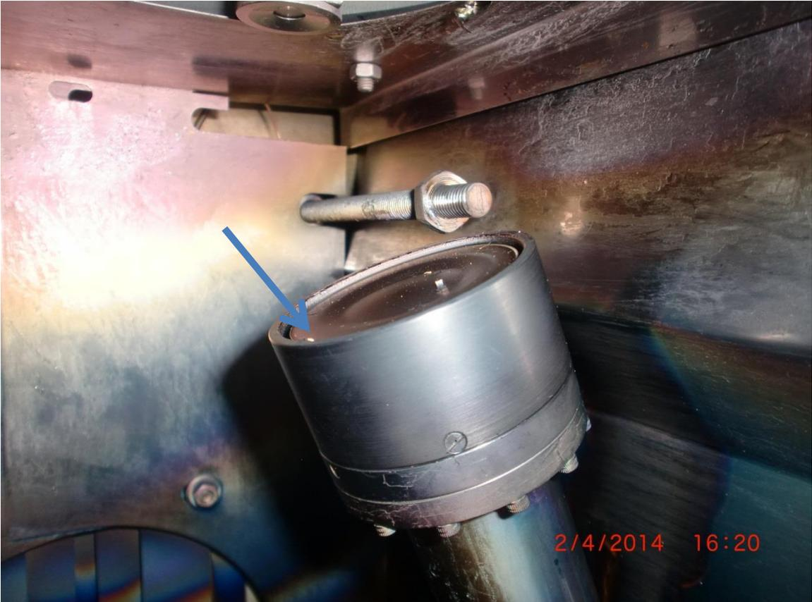
Figure 103 – target with DC sputter head and removed target shutter
