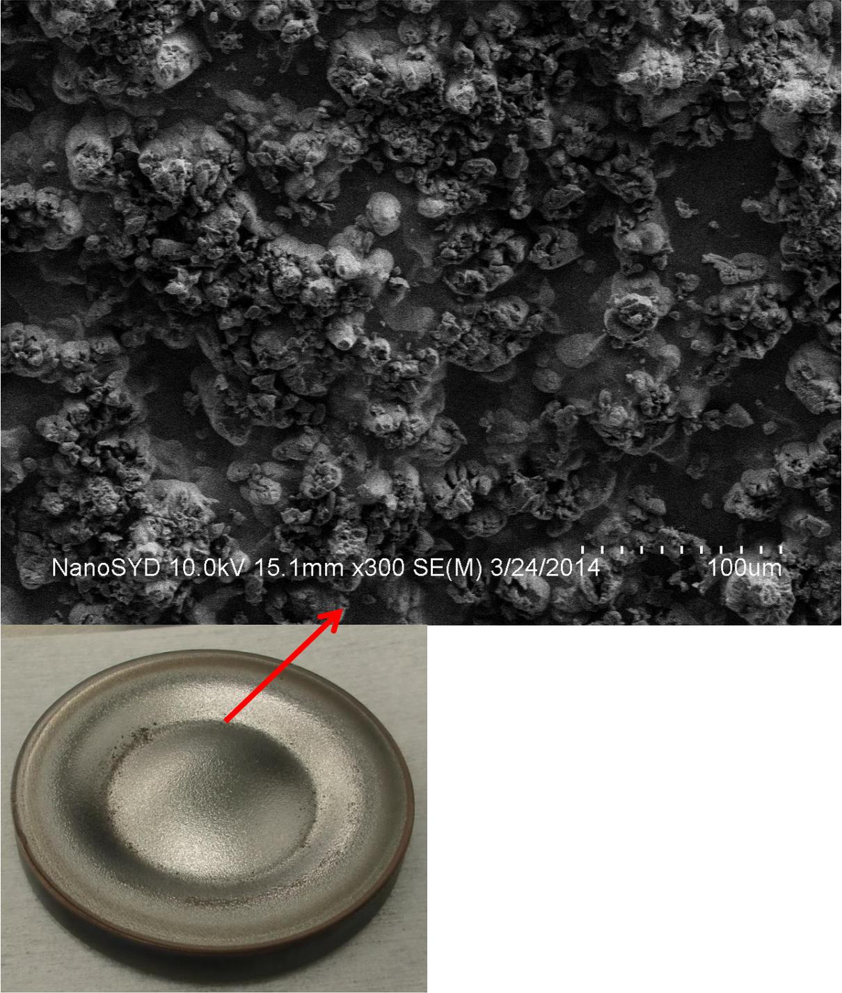
Figure 145 – SEM image of racetrack (upper image) and image of titanium target (lower image)
