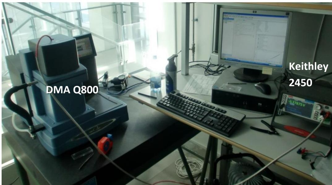
Figure 90 – DMA connected to source meter (Keithley 2400) via high temperature cable. The DMA is controlled via the PC.
