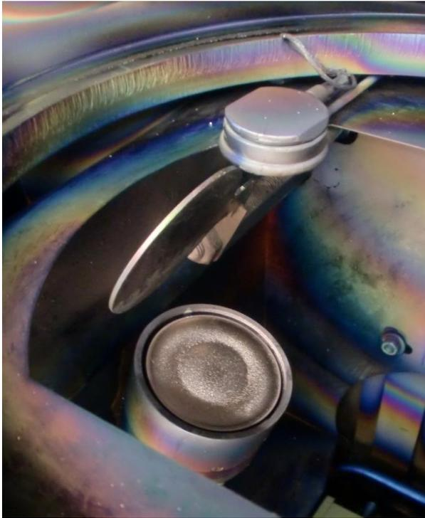
Figure 108 – target shutter top-view
