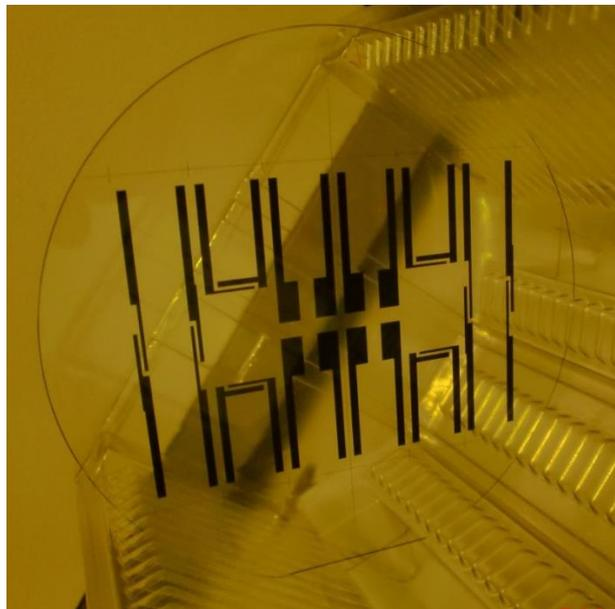
Figure 167- Example of high resolution thin film lithography mask: bottom contacts pattern
