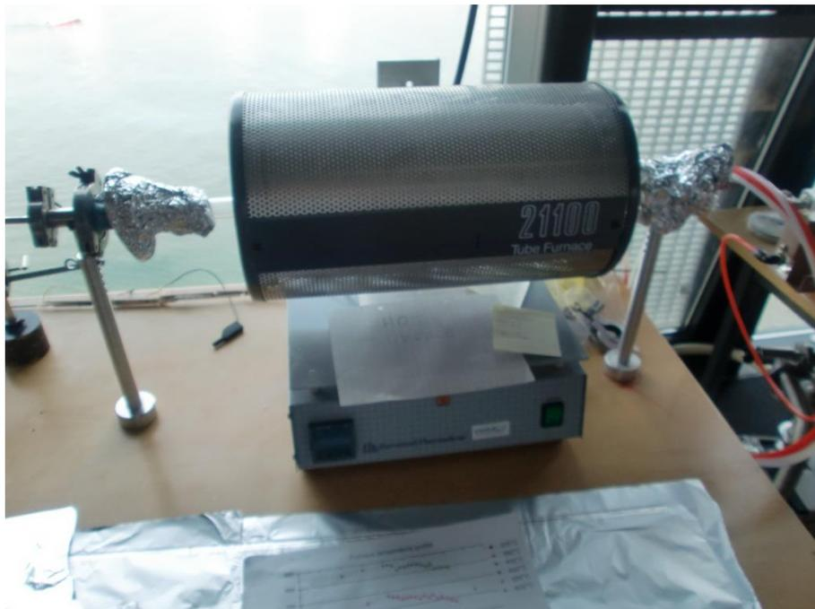
Figure 128 – tube furnace setup connected to argon bottle via red tube
