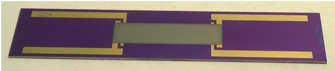
Figure 92 – Longitudinal bottom contact - example sample for gauge factor measurements
