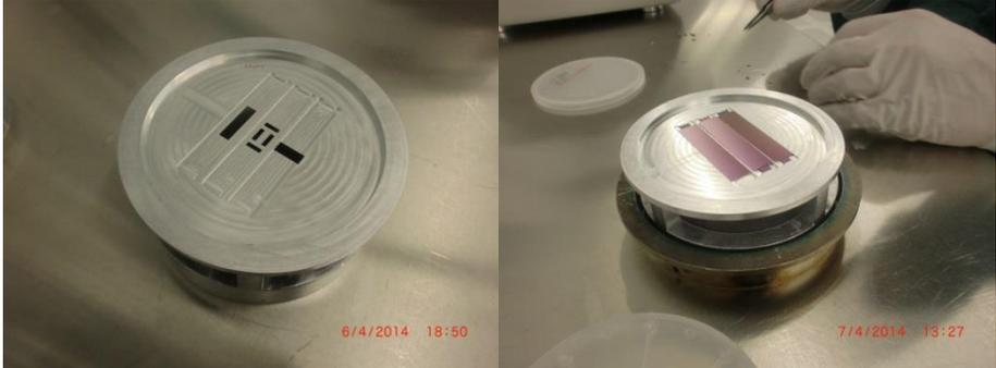
Figure 168 - Shadow mask for the cryofox deposition system
