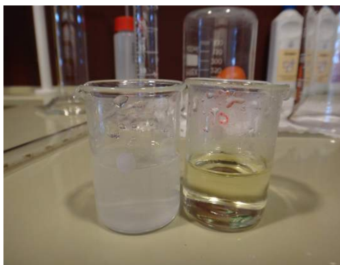
Figure 2-9. Image of cadaverine mixture with different solvent. Left beaker: 10ml water+0.25ml cadaverine; right beaker: 10ml glycerol+0.25ml cadaverine
