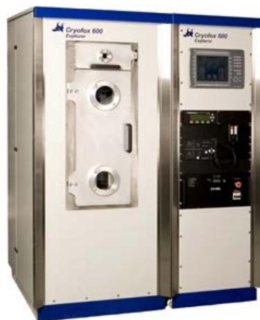
*Figure 2.1 Polytechnik Cryofox Explorer 600 e equipment at NanoSYD used for E-Beam Evaporation of titanium and gold [8].*
