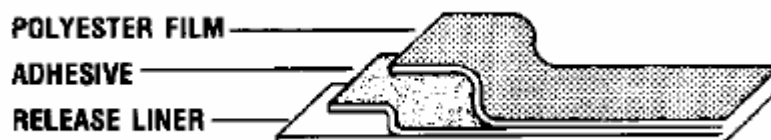
Figure 3-14 – ARcare 7815 polyester tape structure
