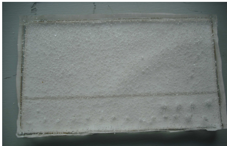
Figure 3-18 – PDMS connector block with holes drilled for a row of connectors in the bottom
