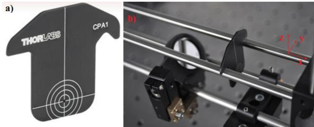
Figure 26 The alignment target (a – picture from datasheet) and presentation of principles of adjusting process (b).
