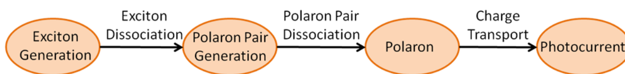
Figure 13. The sketch is illustrating the steps that a photogenerated exciton follows in an organic solar cell, from the generation of the exciton to the production of photocurrent.
