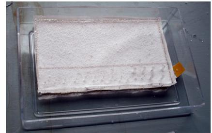
Figure 2.2.4: PDMS ready for cutting off connectors
