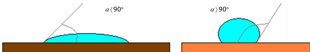
Figure 2.2.2: Left is a water droplet on a hydrophilic material; right a water droplet on a hydrophobic material
