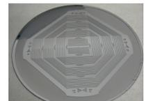
Figure 3.1.16: Wafer without resist
