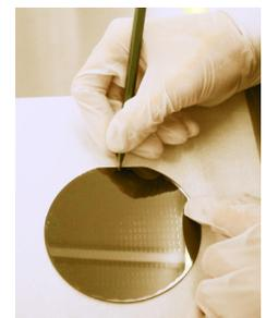
Figure 3.1.17: Cutting of a wafer
