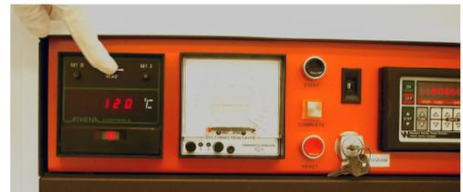
Figure 3.1.6: HMDS oven ready for work
