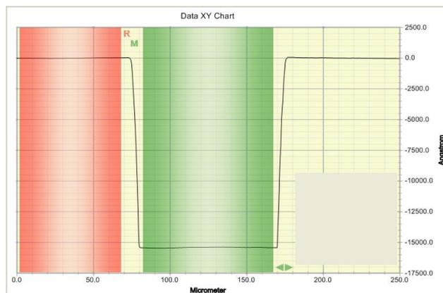
Figure 3.1.11: Resist measurement on profilometer
