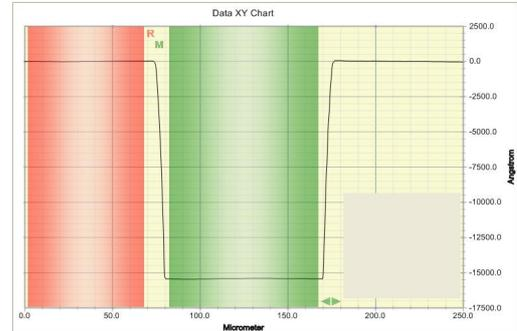
Figure 2.3.9: A picture of resist thickness taken with the profilometer.
