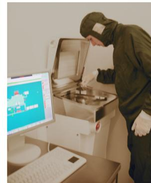
**Figure 3.1.12: Mounting a wafer in the ICP RIE**
