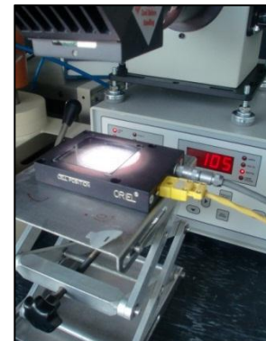
Figure 46 - measurement setup for reference solar cell
