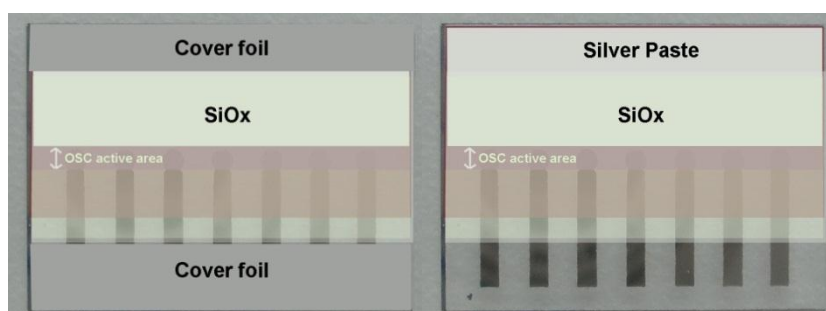
Figure 74 - (left) Sample after the \text{SiO}_x film deposition, (right) finished sample with removed cover foil
