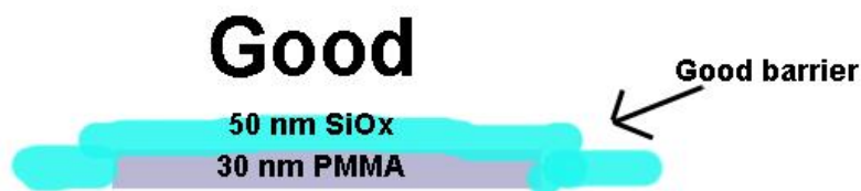
Figure 85 – Side wall coverage - good encapsulation
