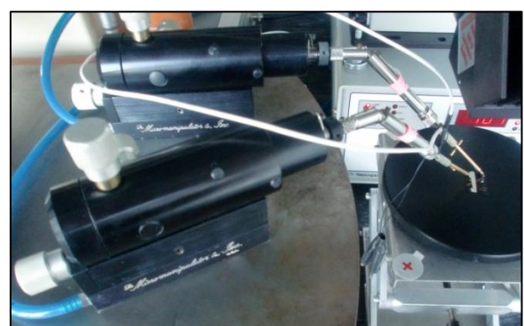
Figure 47 - measurement setup for measuring OSCs
