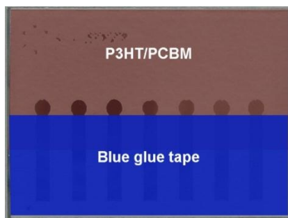
Figure 39 – blue glue stripe controlling solar cell size
