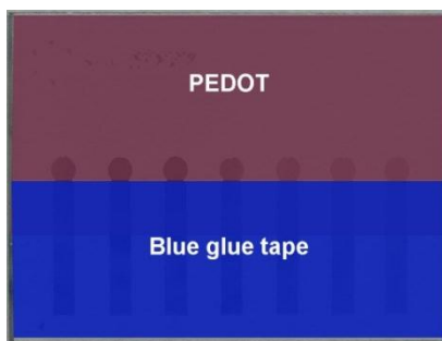
Figure 40 - deposition of PEDOT
