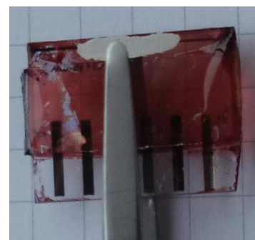
Figure 61 - glass plate / epoxy encapsulation
