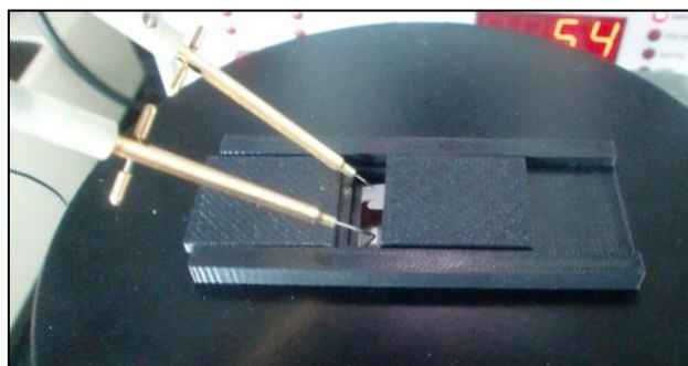
Figure 55 - Printed light shutter in action
