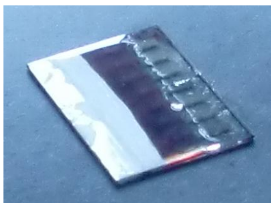
Figure 90 - OSC encapsulated with adhesive
