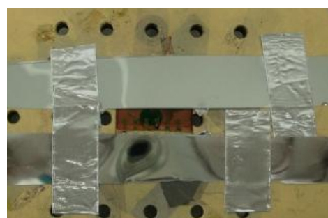
Figure 73 –cover foil applied to the Cryofox sample holder
