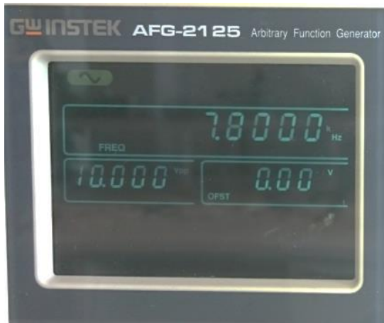
Figure 20: Function generator, emitting a sine wave of 7.8 kHz, 10 V pp
