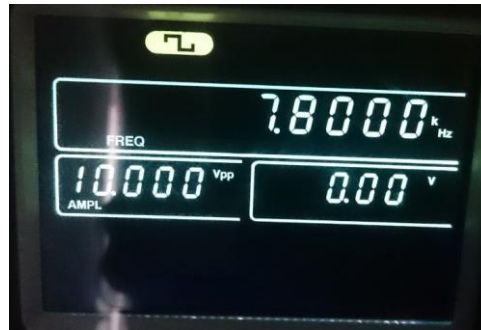
Figure 47: Signal generator setup to drive the piezoelectric beam
