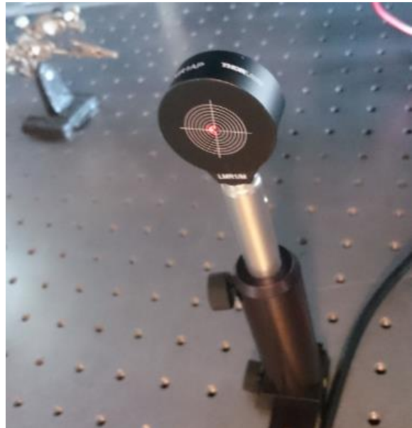
Figure 29: Calibration of laser beam position, so it would cross the central position of each lens.
