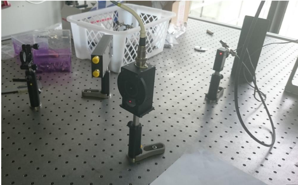
Figure 25: Beam cutter unit running at 1kHz (centre front). Photodiode unit with laser spot on sensitive area (right side)
