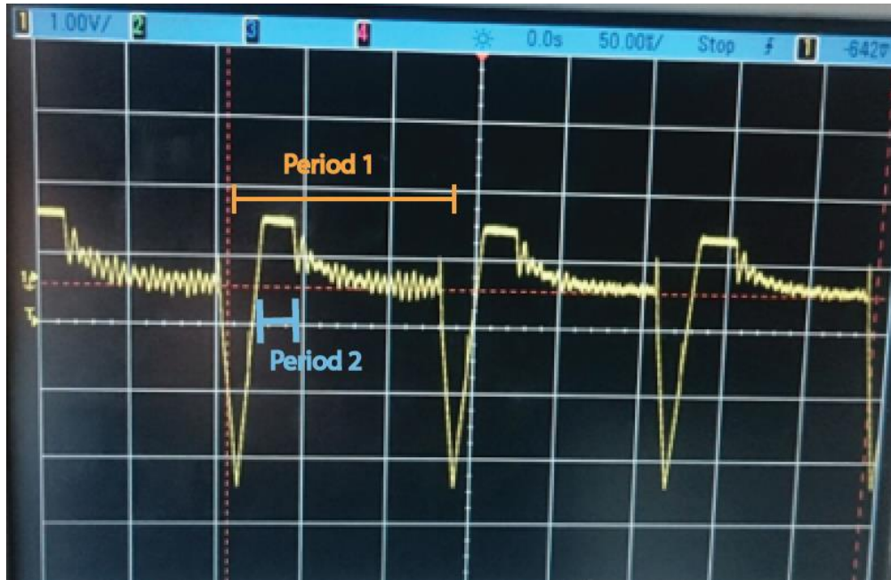
Figure 50: Output signal read in oscilloscope for functionalized cantilever chip. It is noted that the behaviour is quite different from the one obtained in previous testing as seen in Figure 45.
