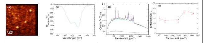
Example of surface enhanced Raman microscopy (a), spectroscopy (c), reflection spectrum (b), and relative enhancement of the Raman peaks (d) for a structure with 100 nm diameter gold particles relative to a flat gold surface [1].
