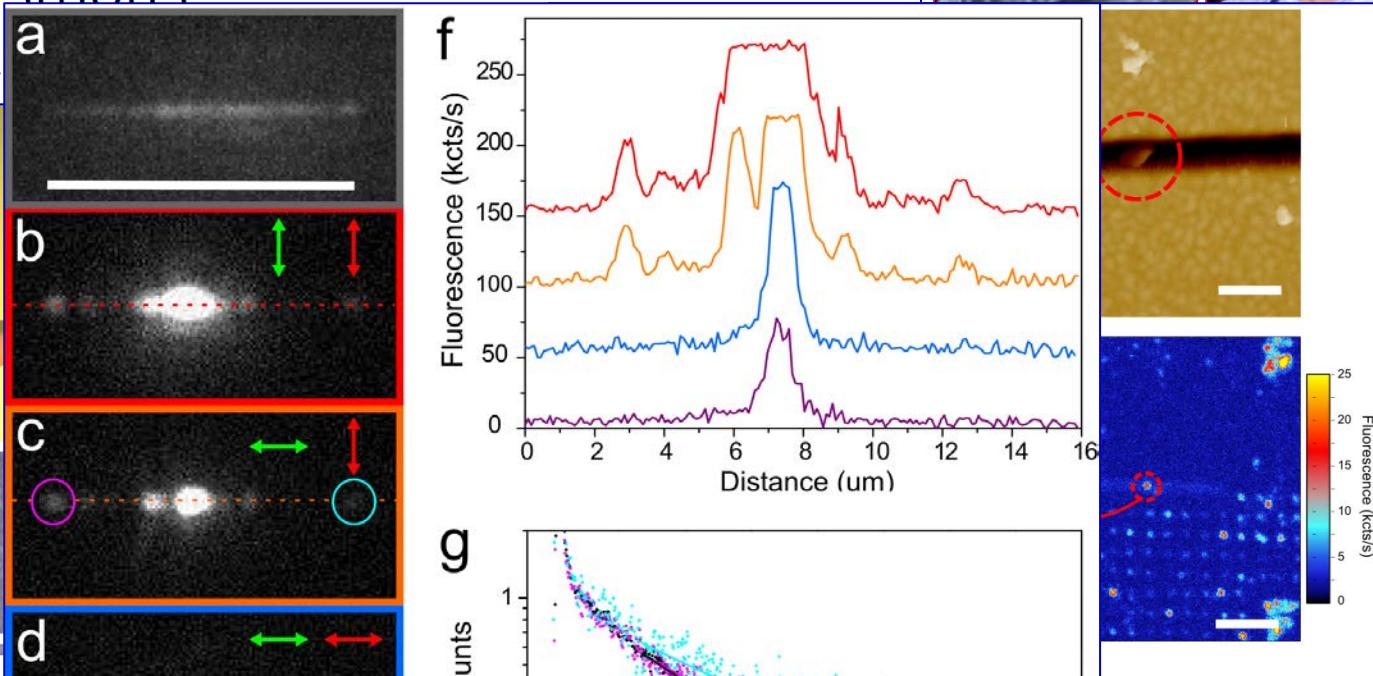
The combination of the  $\beta$ -factor of 0.42, Purcell factor of 2.3 along with propagation length of  $4.65 \mu\text{m}$  normalized by the operating wavelength of  $0.68 \mu\text{m}$ , makes the demonstrated configuration one of the best in terms of FOM ( $6.6 \pm 1.5$ ).
