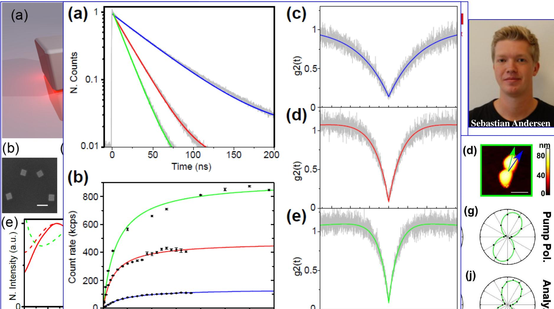
Bright (850 kcps) pure single-photon ( $g^{(2)} \sim 0.08$ ) linearly-polarized sources are demonstrated!
