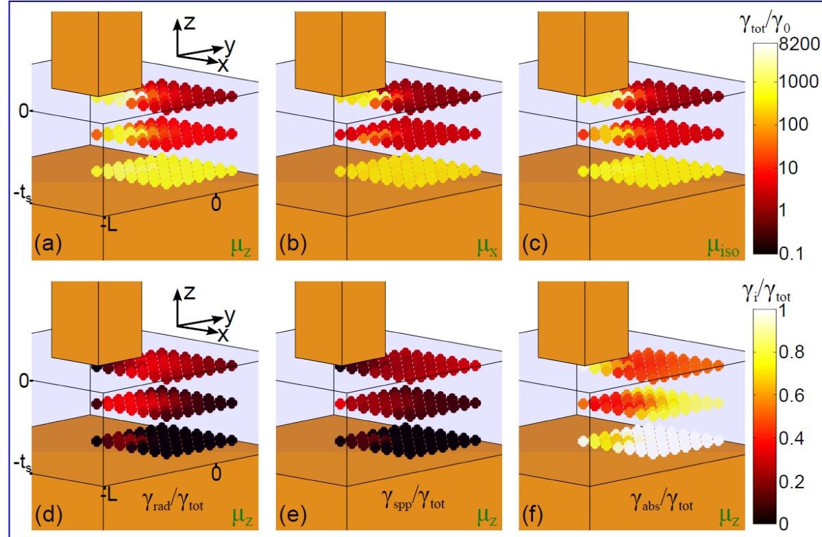
Total decay rate modification for (a) z-directed, (b) x-directed, and (c) isotropically
