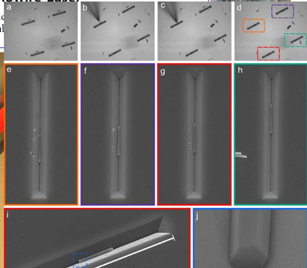
Accurate AFM-based assembly of hybrid NW-VG devices!
