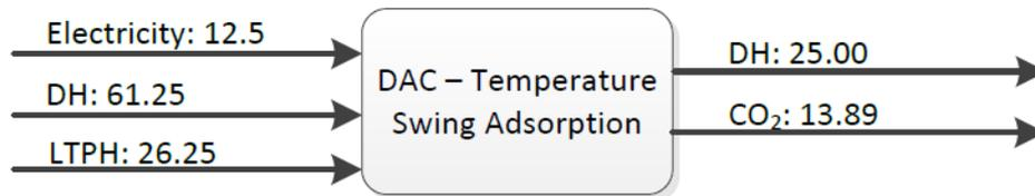
Figure 54 - Net energy balance for temperature swing adsorption of direct air capture of CO<sub>2</sub> [101].
