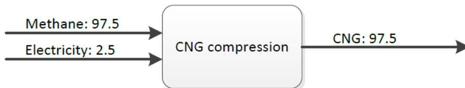
Figure 62 - Net energy balance for compression of methane to CNG [3], [185].
