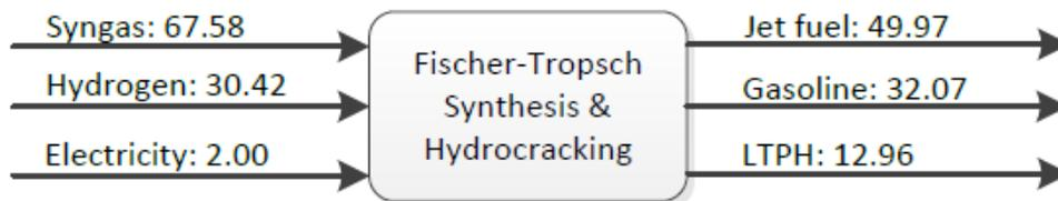
Figure 60 - Net energy balance for FT synthesis with H<sub>2</sub> from water gas shift reaction.
