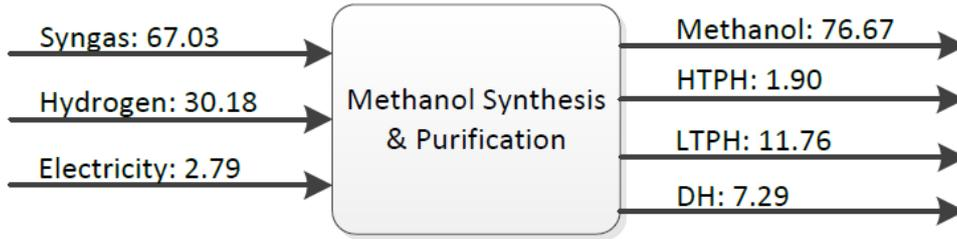
Figure 57 – Net energy balance for methanol synthesis and purification [91].
