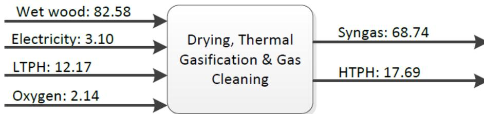
Figure 48 – Net energy balance for the dryer unit, thermal gasification and gas cleaning [91].
