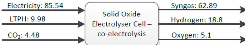
Figure 56 - Net energy balance for solid oxide electrolyser cell for production of syngas [14].
