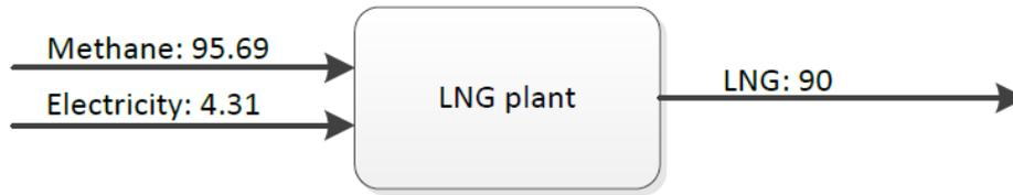
Figure 61 – Net energy balance for liquefaction of methane to LNG [182].
