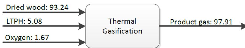
Figure 46 - Net energy balance for thermal gasification[91].
