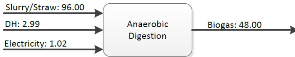
Figure 49 - Net energy balance for anaerobic digestion [162], [163].
