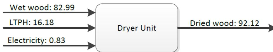
Figure 45 - Net energy balance for the dryer unit [91].
