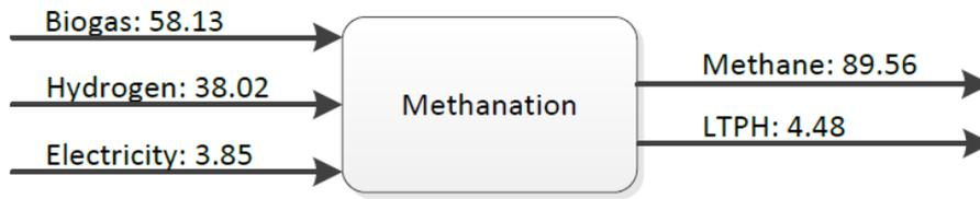
Figure 51 - Net energy balance for methanation of biogas [165]–[167].
