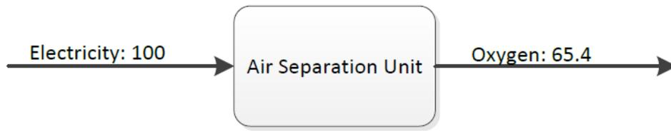
Figure 63 – Net energy balance for the air separation unit [91].
