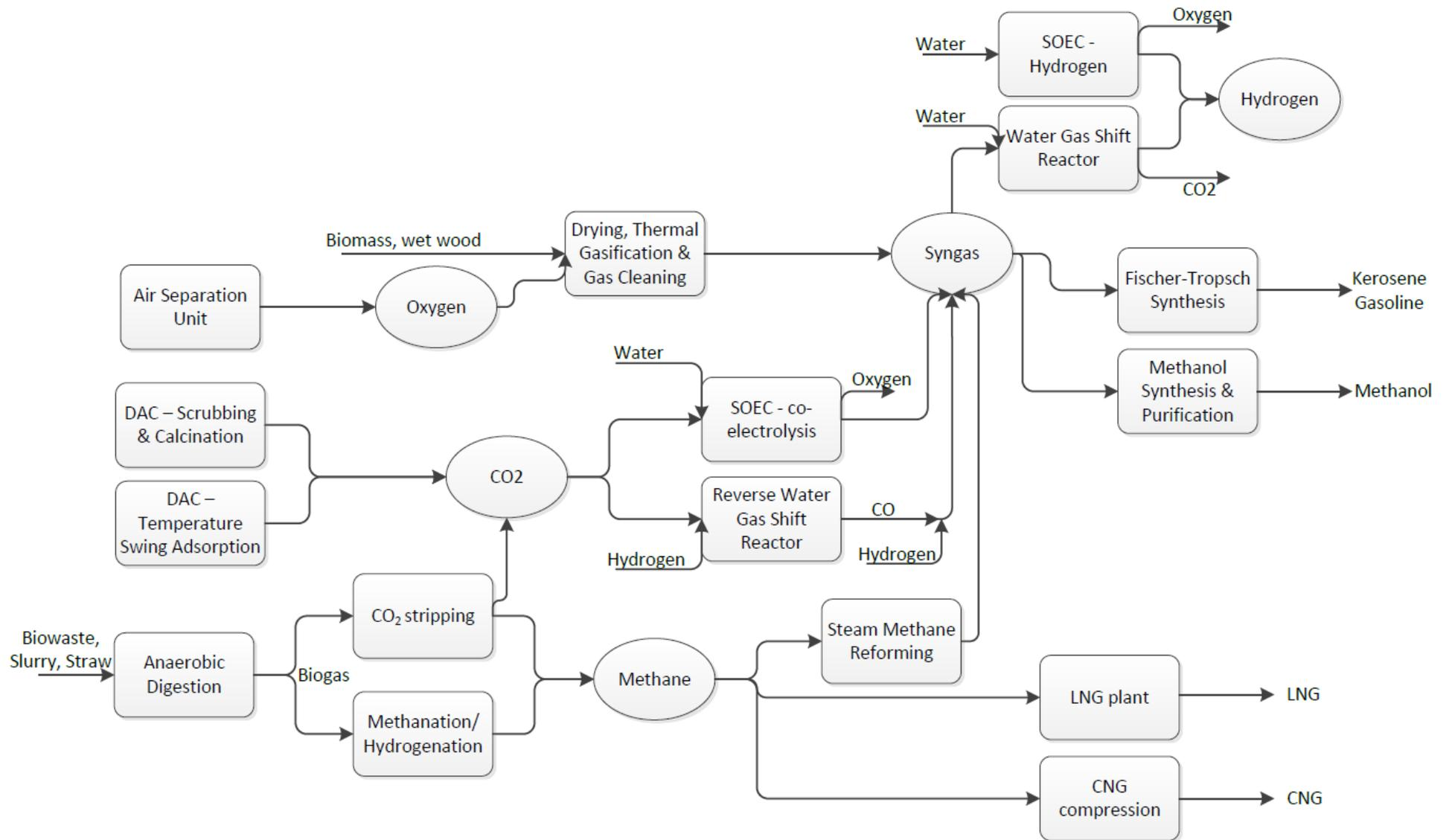
Figure 14 - Overview of the fuel production pathways included in the modelling. Electricity and heat streams are not included in the figure. A more detailed version including all streams and connections to the heat and power system can be found in Appendix G – Sifre Modelling of Fuel Production Pathways.
