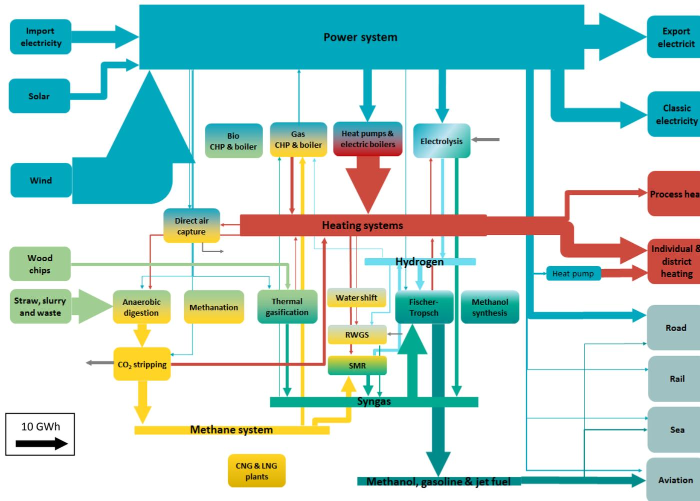
Figure 23 - Sankey diagram illustrating energy flows for DG "Moderate". CO<sub>2</sub>-streams are based on the arbitrary LHV of 1 MJ/kg and scaled by a factor ten. The RWGS unit in the Sankey diagram includes the mixing of the CO with hydrogen to form syngas.
