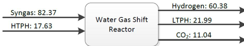
Figure 58 - Net energy balance for water gas shift reactor [91].
