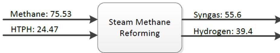
Figure 52 - Net energy balance for steam methane reforming [94], [164].
