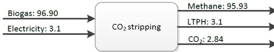
Figure 50 - Net energy balance for CO<sub>2</sub> stripping of biogas [161].
