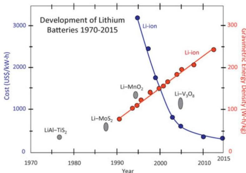
Figure 11 – Development of cost and energy density of lithium batteries [57].
