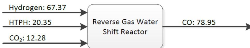
Figure 59 - Net energy balance for reverse water gas shift reactor [174], [175].
