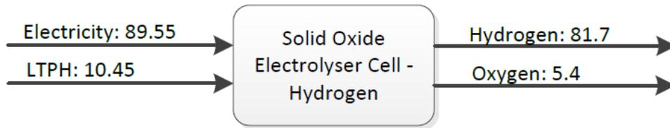
Figure 55 - Net energy balance for solid oxide electrolyser cell for production of hydrogen [14].
