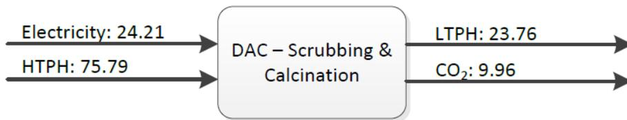
Figure 53 - Net energy balance for scrubbing and calcination of direct air capture of CO<sub>2</sub> [171].
