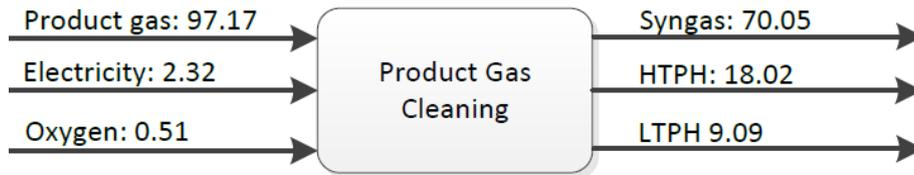
Figure 47 - Net energy balance for the gas cleaning process after thermal gasification [91].
