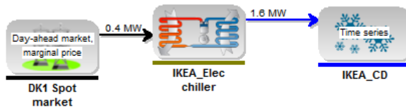
Figure 15.1 IKEA site in energyPRO. The two 750 kW electrical chillers are combined to one called IKEA_Elec chiller. The IKEA_Elec chiller by electricity from the DK1 spot market. The cooling demand (IKEA_CD) is based on hourly cooling demand data from Fjernvarme Fyn.
