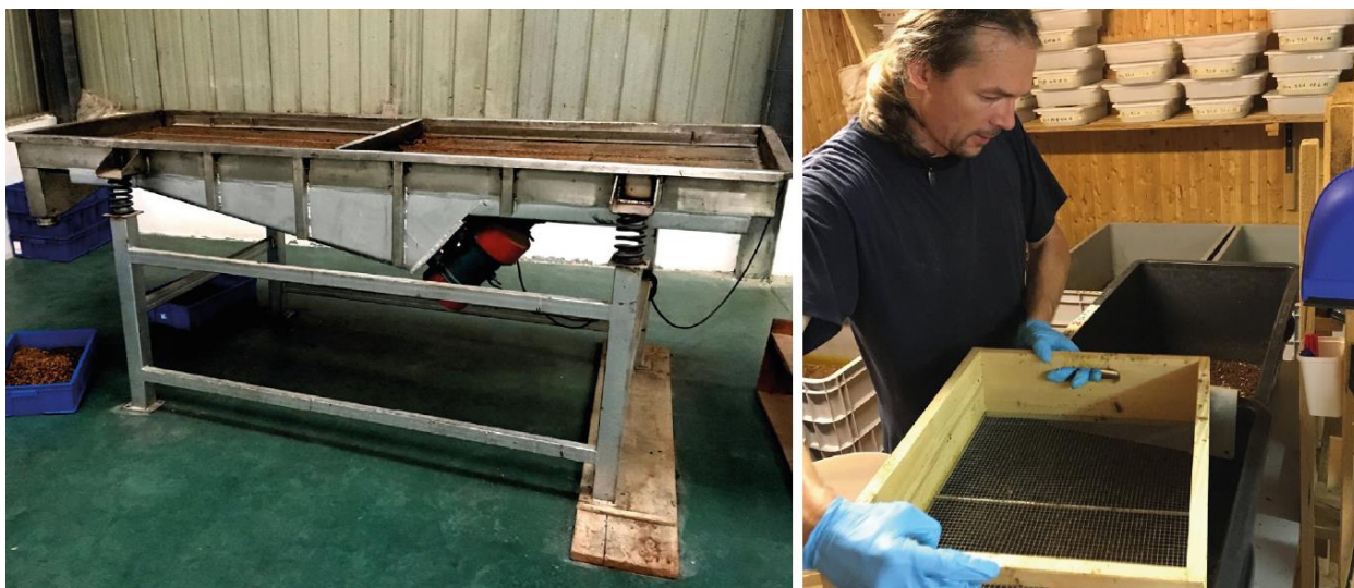
Figure 23: Automated shaking sieve on the left side, manual sieve on the right side (Dortmans B.M.A. 2017)
