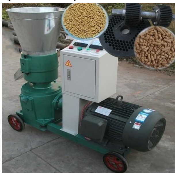
Figure 24: Pelletizer for animal feed
