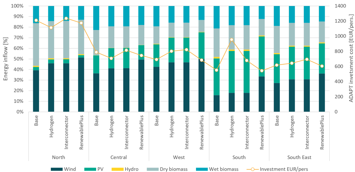
Figure 22: The figure shows the fuel inflow and yearly investment costs across Europe in the four scenarios. The inflow in the energy system consists of renewable production units along with biomass resources. The wet biomass is used in the anaerobic digestion process. Dry biomass is used in the thermal gasification process, along with bio CHP and boiler units. The yearly investment cost is given per person in the clusters.
