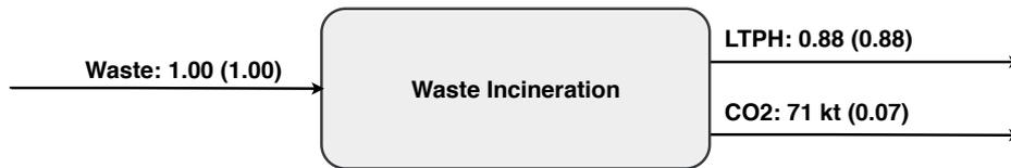
**Figure B.11:** Energy balance of waste incineration [72]. The energy balance includes a carbon capture rate of 75% [47], while the actual content of  $CO_2$  is approximately 95 kt/PJ.
