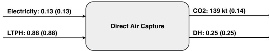
**Figure B.10:** Energy balance of temperature swing adsorption direct air capture [13].
