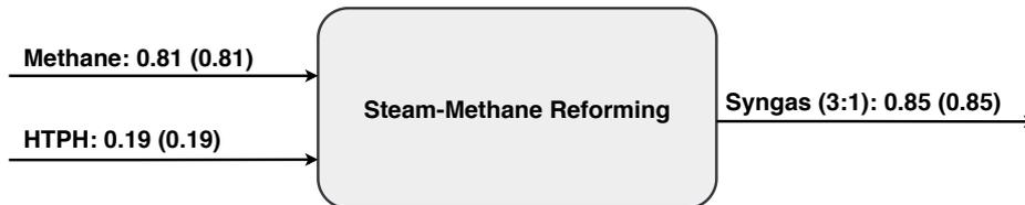
Figure B.3: Energy balance of steam-methane reforming [21].
