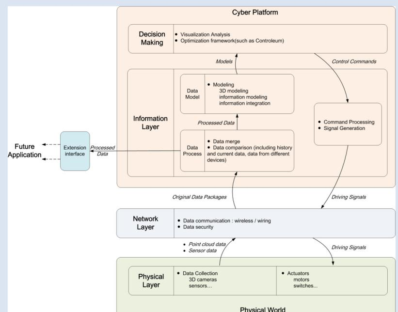
Figure 1 Architecture of the Digital Twin System for the PhD project.
