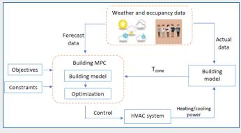
Fig. 1. Example of building MPC (T<sub>zone</sub> is temperature in specific building zone)
