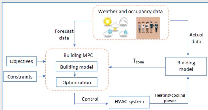
Fig. 1. Example of building MPC
