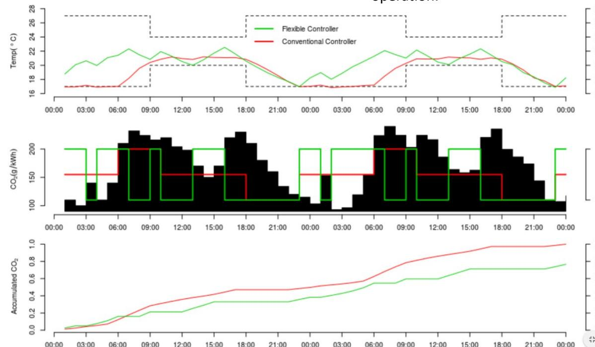
Example on demand-side flexibility using the thermal mass of a building. The conventional controller minimizes electricity usage while flexible controller minimizes CO<sub>2</sub>-emissions [1].
