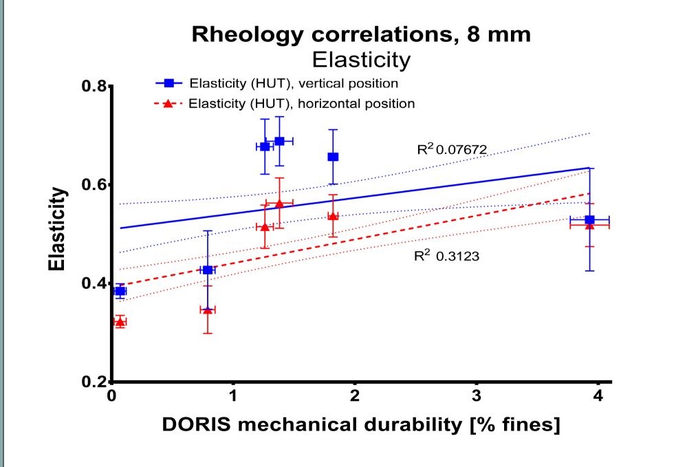
The 'elasticity' of a pellet is found to have some importance. Pellets will have a high durability when able to relax the force applied at the surface as deformations in non-elastic type behavior.
