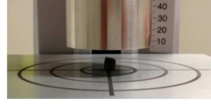
Force exerted against the weigh cell is recorded over time and can be used for graphical analysis.
