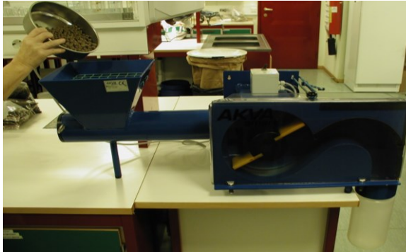
Fig. 1: The DORIS tester comprising an inlet grid, a screw conveyor, a rotating fan and a sample collector bin (EWOS Innovation 2003)
