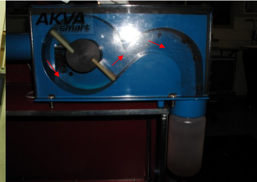
Fig. 2: The feed pellets are accelerated into a wall and collected for sifting analysis (EWOS Innovation 2003).
