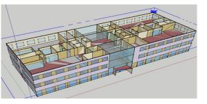
Based on the Revit BIM model, an E+ model has been developed. An ideal load energy plus performance simulation of the building has been completed and pre-tuned. The model needs to be upgraded by implementing the accurate energy supply system characteristics and specifications. In addition zone models have been developed and preliminary testing is underway.
