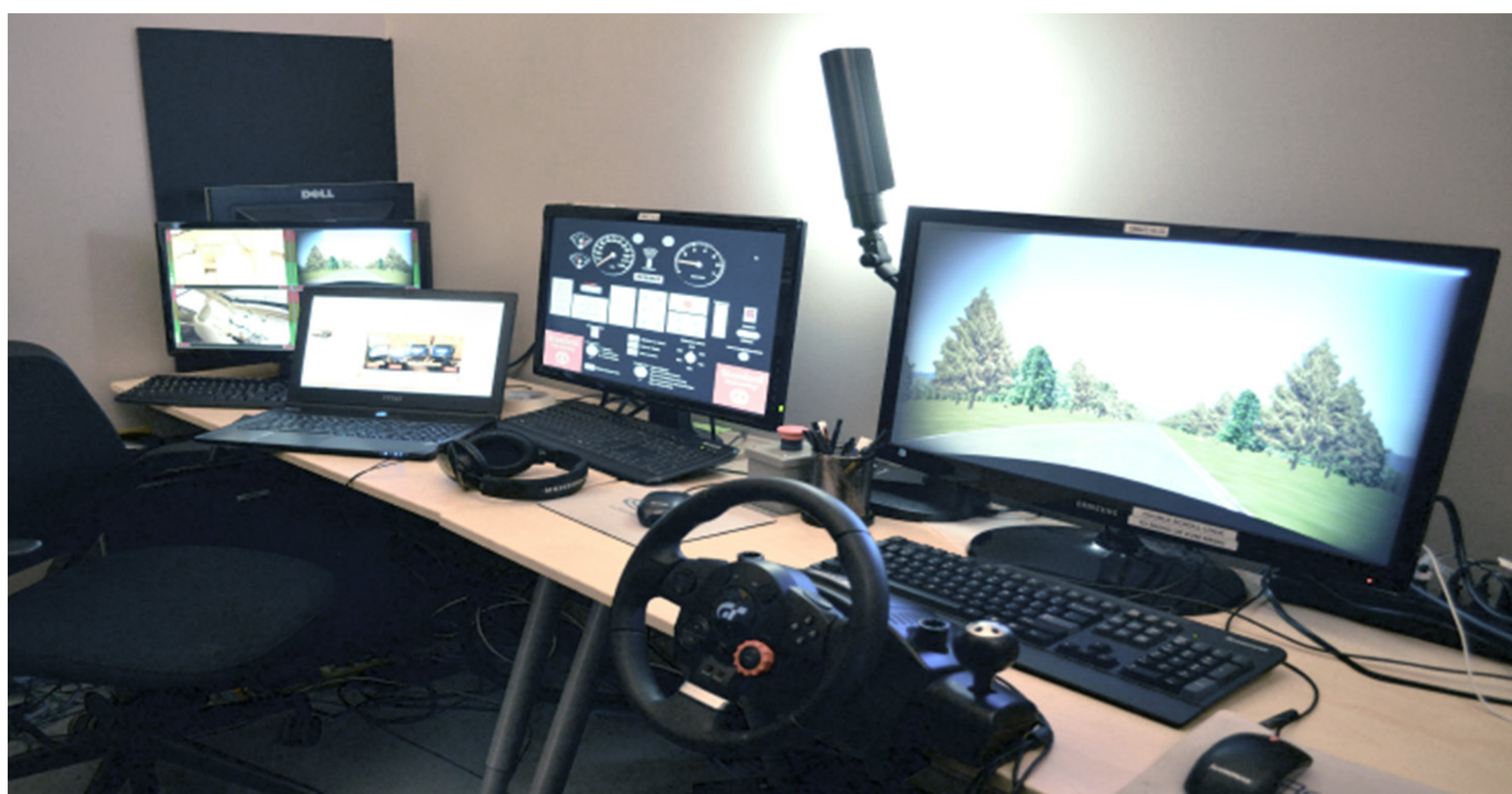
We use a 2-Wizard setup to simultaneously interact with drivers and control the car.
