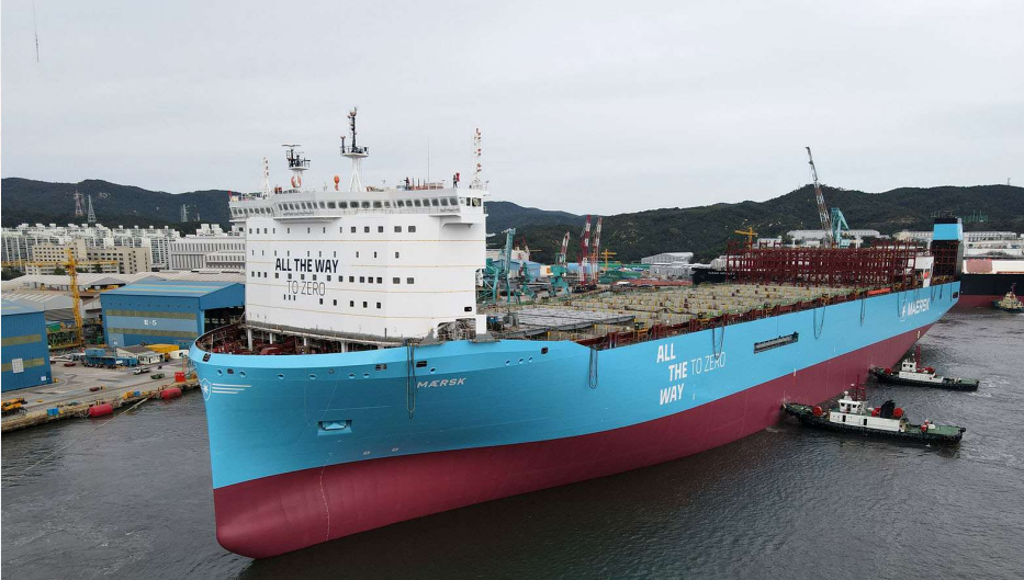
The first in a series of 12 methanol containerships launched in the water Oct 2023. 16,200 TEU.
