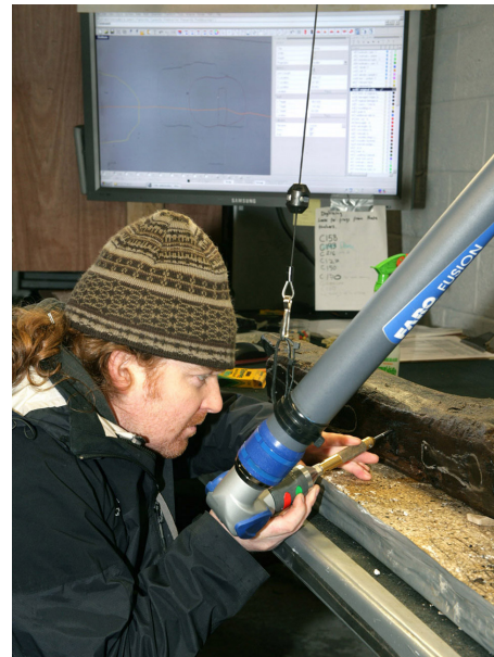
Figure 3-4: FaroArm recording (Brogan 2009)
