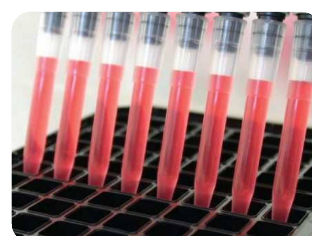
Figure 7: Example of 96-well plate with sample pipettes, used for automating preparation, transport and processing of multiple samples in an efficient way.
